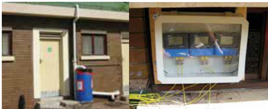
Measuring rainfall run-off and energy use (Van Niekerk et al 2011)
